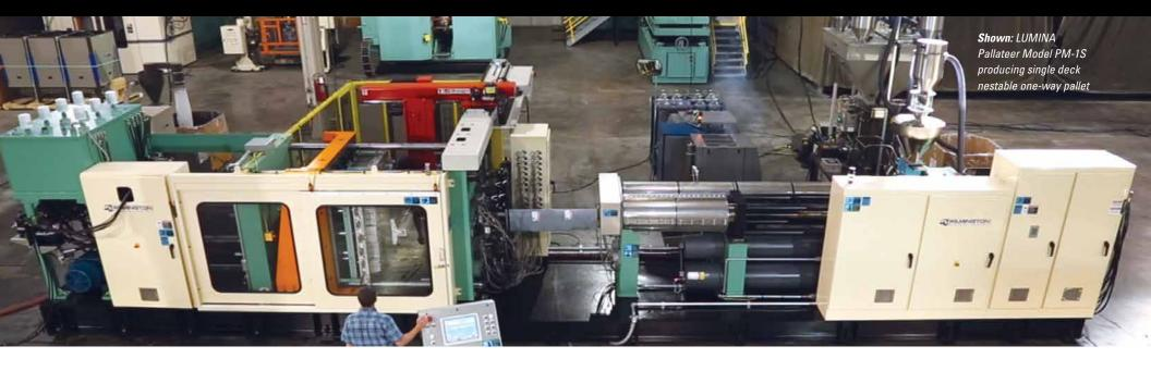
Wilmington Machinery has built structural foam injection molding machinery for since 1972. This method of molding has proven to be the most successful in the making of plastic pallets. Alternatively, the gas assist method of molding can be applied on the same machinery.
